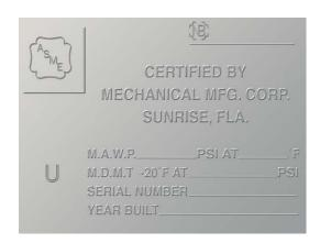
**ASME Code Nameplate** identifies both the National Board Number and the Serial Number of the vessel. A "U" Stamp indicates that the Vessel has been designed and manufactured in accordance with the guidelines of ASME Code Section 8. Division 1. Limits of safe working pressures and temperatures are designated on the nameplate.
